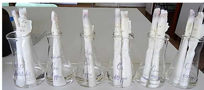
Fig. 2. Germination rolls treated with distilled water for control and graded solutions for Cu: 1ppm, 10 ppm, 50 ppm, 100 ppm
