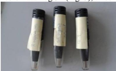
Fig. 3. Data Logger LOG 32
