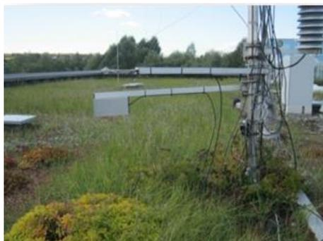
Fig.4. LOG 32 placed on 50 cm above the green roof
