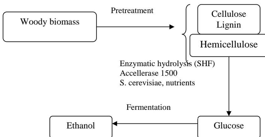
**Fig.1. Schematic presentation of the procedure to convert wood to ethanol**
