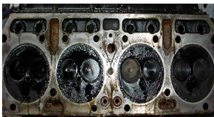
Fig. 5. The bio-diesel influence over the head of piston
