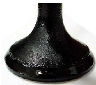
Fig.4. The bio-diesel influence over valve
