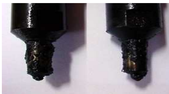
Fig. 3. The bio-diesel influence over injectors
