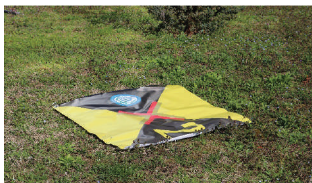
Figure 15. Ground markers used for georeference
