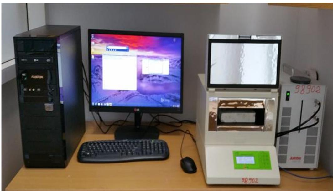
Figure 5. The thermal conductivity measuring device
