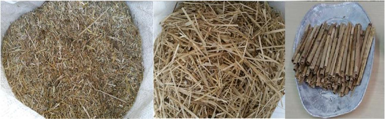
**Figure 3.** The fibres used in the experimental activity from left to right: ground straw, ground reed and reed strips
