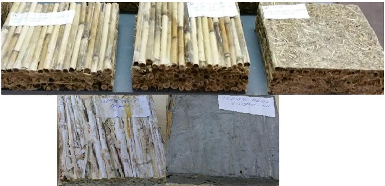
**Figure 4.** Straw and reed-based thermally insulating panels
