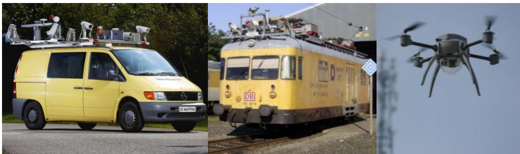
Fig. 3 - mobile scanning systems, from left to right: Moses, Rail Mapper, MicroDrone
