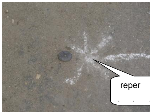
Fig. 2. Reper de nivelment Leveling landmark
