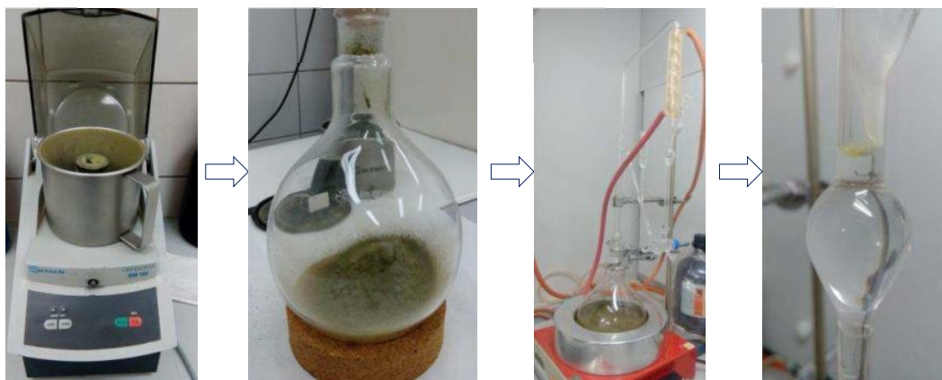
Figure 2. Hydrodistillation process of plant material using a Clevenger-type apparatus
