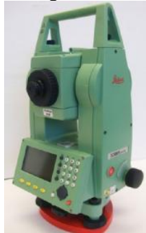
Fig 2. Leica TCR 805 total station
