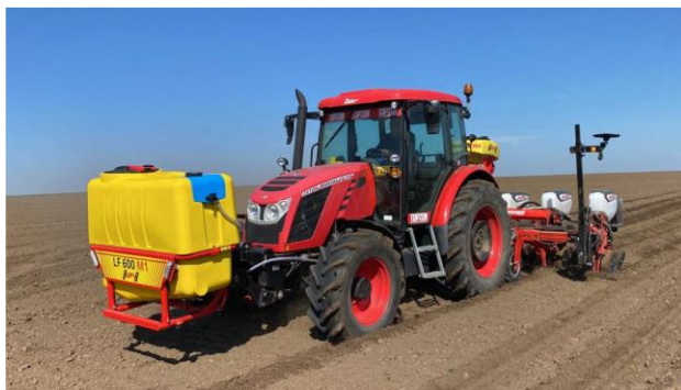
Figure 4. Example of an aggregate composed of tractor, seeder and liquid fertilizer applicator [original]
