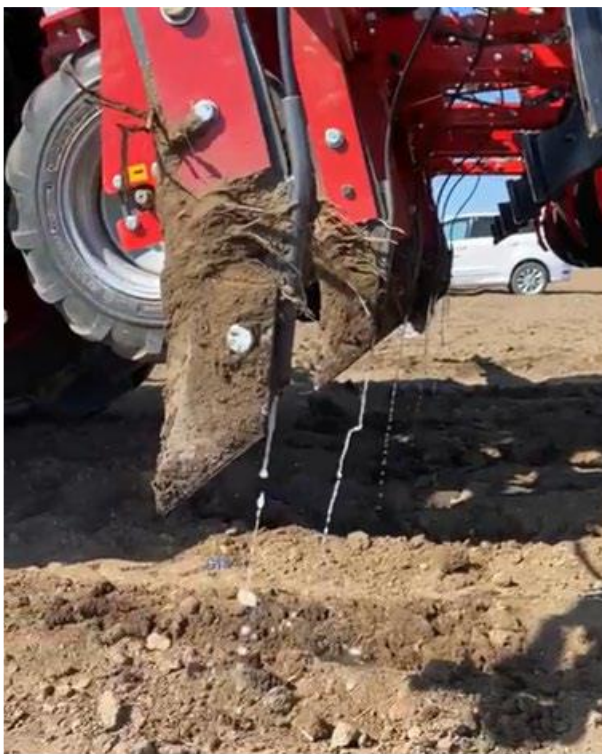
Figure 10. Example of injection system for liquid fertilizer [original]
