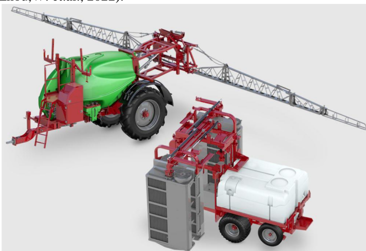
Figure 1. Example of Tow-Behind Sprayer (up) and Mist Blower machinery for vineyard ( https://polmac.it/en/ )
