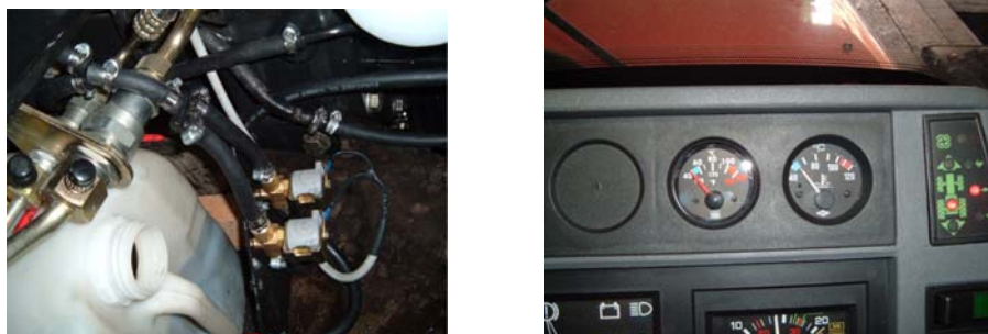
Fig. 4. Left: electronic valves to switch the fuel system from the diesel to the blend tank and vice versa; Right: tractor dashboard with exchanger temperature control and switch button
