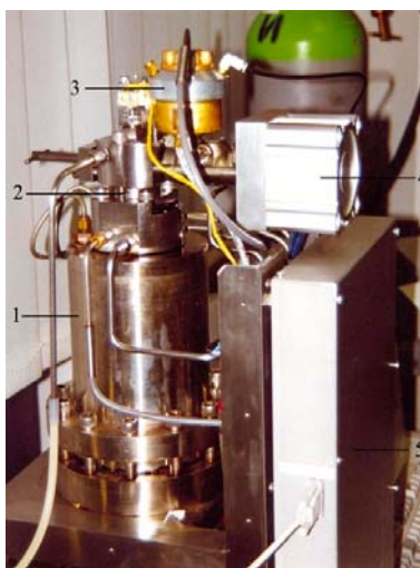
Fig. 2. The apparatus FIA 100; (1) cylinder; (2) injector; (3) fuel tank; (4) high pressure pump; (5) control electronic unit with microprocessor.
