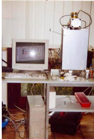
Fig. 1. The stand with FIA 100;(1) the apparatus FIA100; (2)- the unit for data recording (computer).
