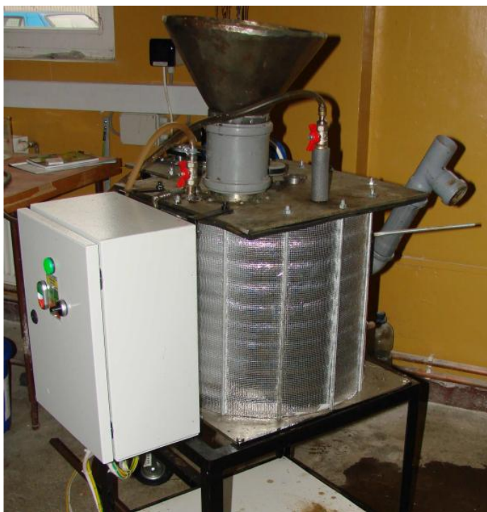
Fig. 1. The experimental anaerobic vertical digester
