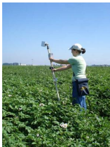
Fig.2 The canopy reflectance monitoring with CropScan multispectral radiometer
