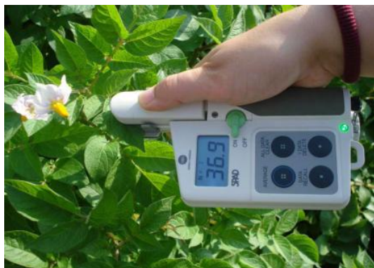
Fig.1 The leaf chlorophyll content monitoring with SPAD 502 Plus Chlorophyll Meter
