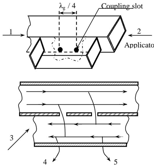
Fig. 7. Directional coupler with two slots:
