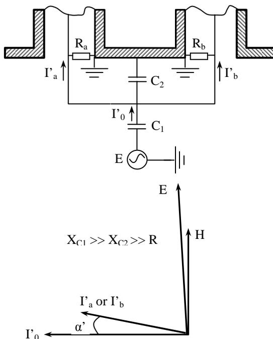
Fig. 6. The equivalent diagram and the vectorial diagram for the currents induced by the electric current.
