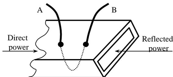
Fig. 4. The currents in the cable „A” are determined by the wave that spreads on the transmission line from left towards right (transmitted power) and the currents in the cable „B” are determined by the wave that spreads from right towards left
