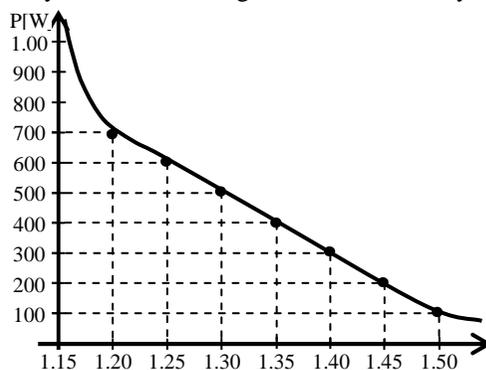
Fig. 1. The output power variation in the microwaves dependMag. field the magnetic field intensity.
