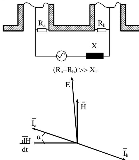
Fig. 5. The equivalent diagram and the vectorial diagram of the currents induced by the magnetic field.
