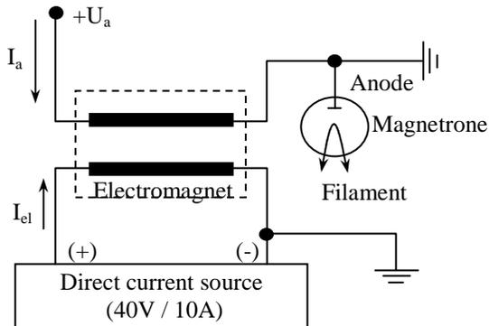
Fig. 2. The electric diagram used for the output power adjustment in the microwaves by adjusting the magnetic field of the magnetron.
