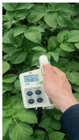
Figure 4. Measuring the chlorophyll content with the SPAD-502PLUS device, on a potato leaf from the experimental field in Rusciori.
