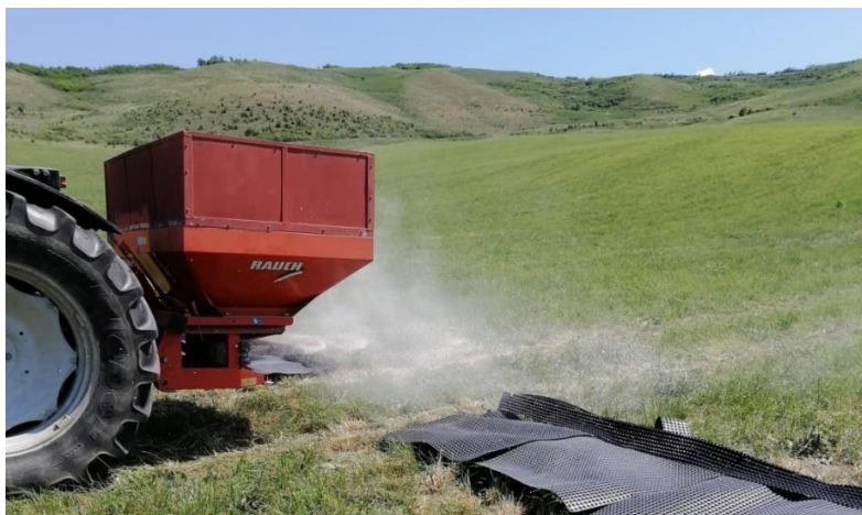
Figure 1. Spreading of fertilizer using the Rauch MDS 935 solid fertilizer broadcaster over the collecting points.
