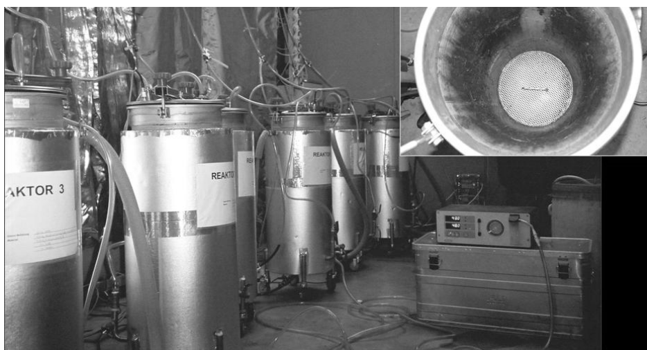
Fig. 1 Solid-phase digestion laboratory at University of Hohenheim
