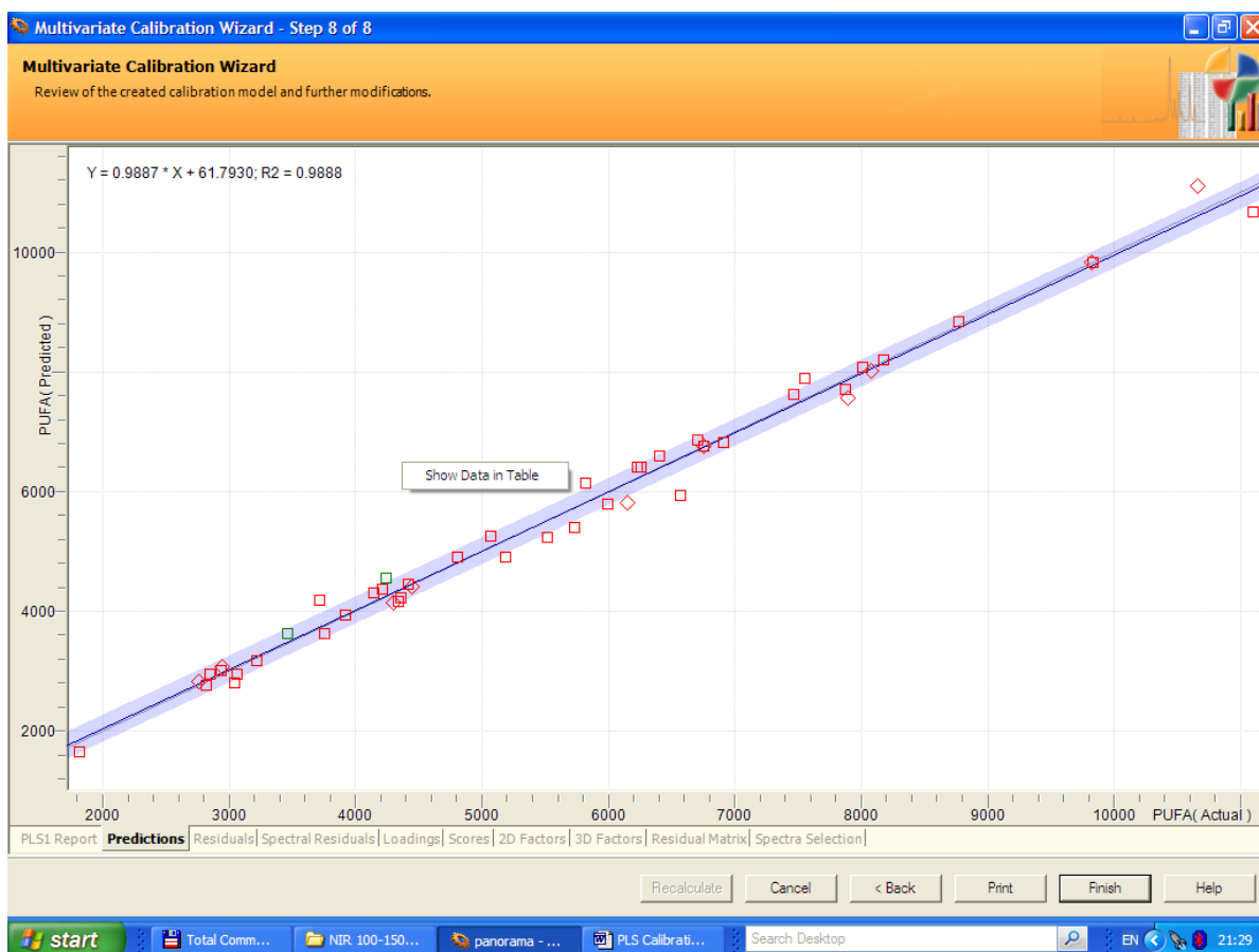
Fig. 1. The NIRS predicted values versus chemical results of PUFAs (mg/kg) on 800 – 2500nm spectral range
