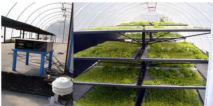
Fig. 1. Instrumentation during no load and inside view of tunnel dryer with product (Rathore and Panwar, 2010)
