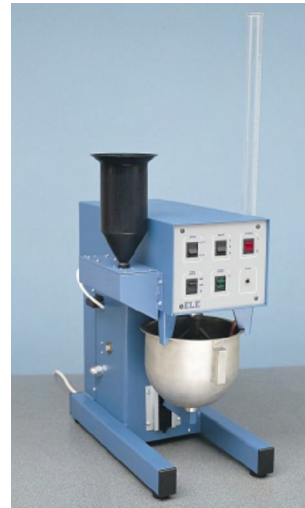
Fig. 2. Automatic standardized mixing device
