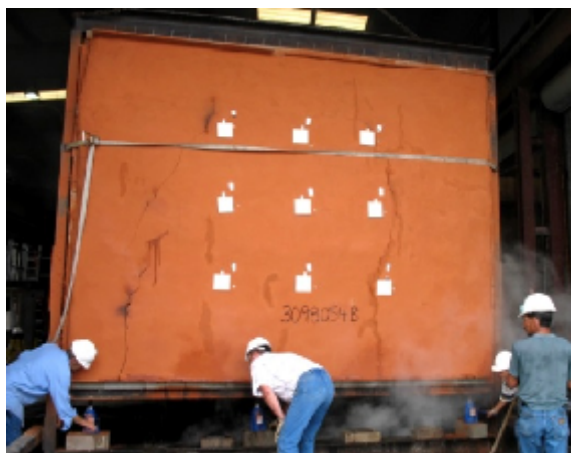
Figure 5 (b). Unexposed part of wall [19]
