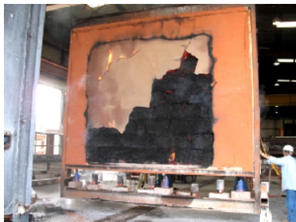
Figure 5 (a). Straw bale wall after fire test [19]
