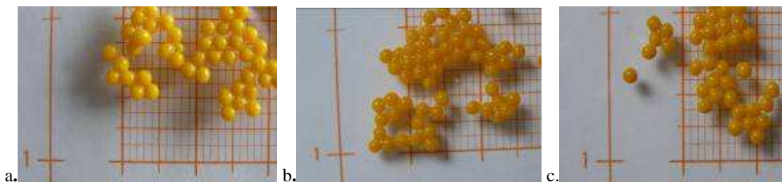
Fig. 2 Sodium alginate beads with sea buckthorn oil: a. 2% w/v. b. 1.5% w/v. c. 1% w/v
